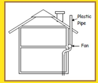
A small fan pulls the radon from the ground into the pipe and out into the air above the roof.
